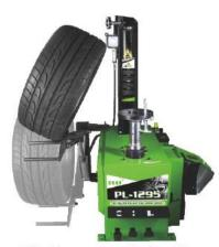
Lift side pneumatic tyre lifter to help easy lift up the tyres, save man-power.
